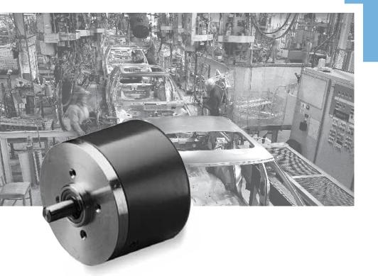
The LD20 incremental encoder, made with a light duty shaft, has an IP50 protection rating. It features a two inch outer diameter, sealed bearings and a quadrature output with a reference marker.
