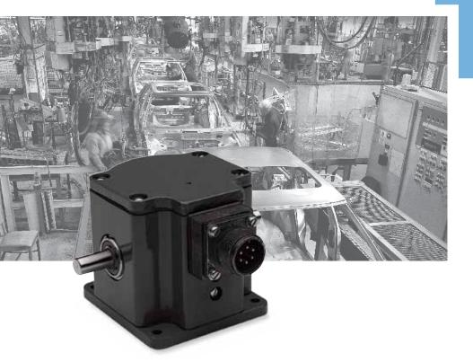
The HD32 is a heavy duty incremental encoder with 100 lb. radial shaft rating. It has a rugged die-cast aluminum housing with IP65 protection. Its double-ended shaft option and quadrature output with reference marker make it an excellent choice for special purpose applications.
