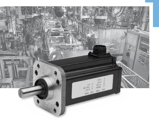
The HD32 is a heavy duty incremental encoder with 100 lb. radial shaft rating. It has a rugged die-cast aluminum housing with IP66 protection. Its quadrature output with reference marker makes it an excellent choice for special purpose applications.
